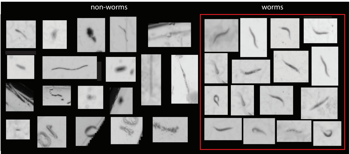
Figure 2-3: Worm and non-worm objects. The images inside the red rectangle exemplify worm objects; the images on the left, outside the rectangle, illustrate various non-worm objects ranging from fibers, to dust, to lot numbers stamped on plates. The two classes of objects are well-separated by the Support Vector Machine, Fig. 2-4, based on the feature set shown in Fig. 2-2.
